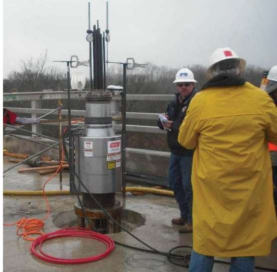
Figure 16. Performance Testing a 20 Strand Tendon
