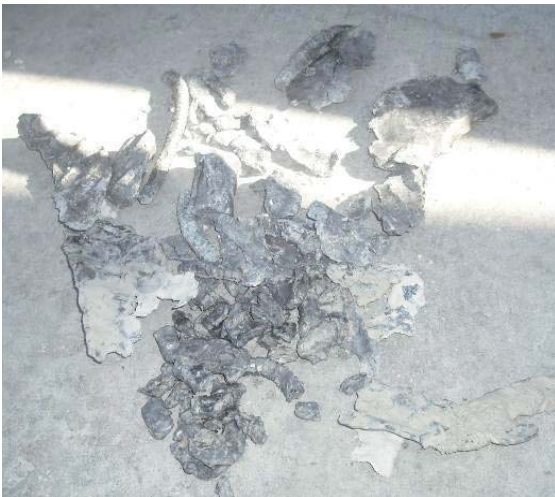
Figure 10. Steel Removed from One Hole
